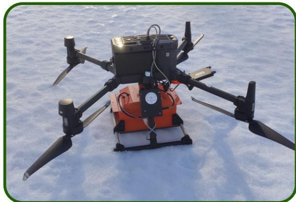
**Zond Aero 1000** is an ultra light weight single-unit GPR, specially designed for portable solutions. Device could be used as the standalone on-board equipment with the powering from external source and Ethernet cable connection or inside of the fully protective case with its own built-in Lithium-Ion battery and WiFi.
